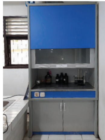
Gambar 4.34 Fume hood. Sumber: Wagiyono/2022
