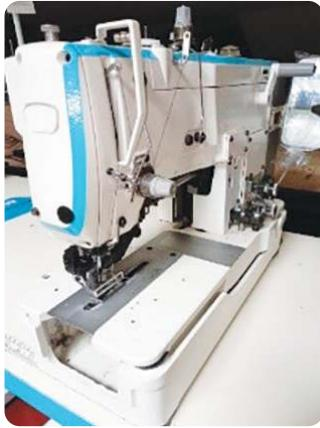
**Gambar 7.8** Mesin Lubang Kancing
