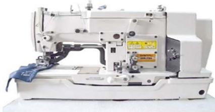
**Gambar 9.11** Mesin Lubang Kancing
