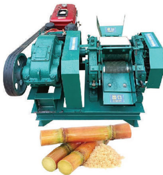
Gambar 4.5 Mesin penghancur batang tebu ( sugar cane crusher ). Sumber: alibaba.com/2023
