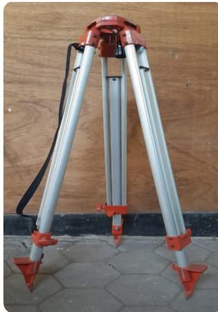
Gambar 4.7 Statif/Tripod
