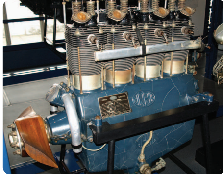
Gambar 2.5 Piston Tipe Satu Garis Sumber: wikipedia.org/Nimbus227 (2011)
