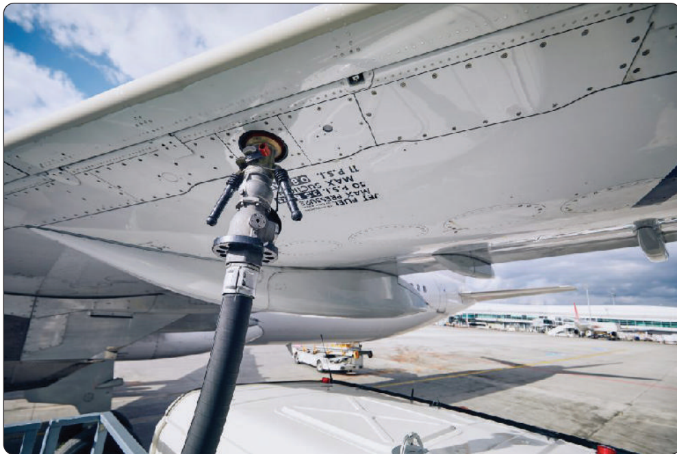
Gambar 4.31 Sistem Pengisian Bahan Bakar Sumber: Shutterstock.com/Jaromir Chalabala (2022)
