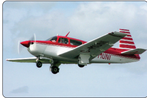
Gambar 4.52 Tricycle Landing Gear
