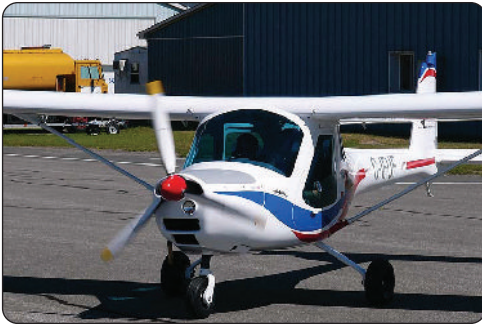
Gambar 4.52 Tricycle Landing Gear
