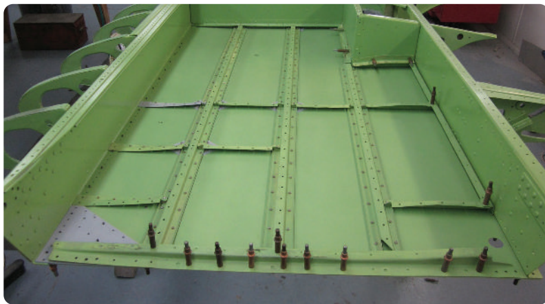
B. The Wing Skin Riveting Process Sumber: rjdauhnaircraft.com (2015)
