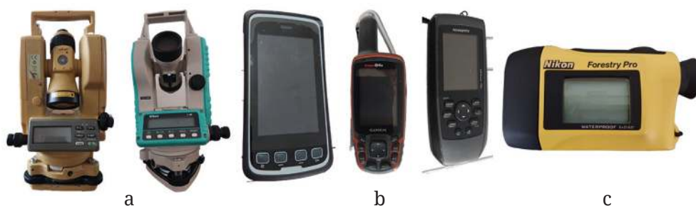
Gambar 3.4 Macam-Macam Peralatan Digital: (a) Teodolit Digital, (b) GPS Receiver , dan (c) Rangefinder .
