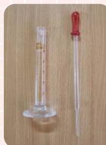
**Gambar 4.2** (a) pipet tetes; (b) gelas ukur
