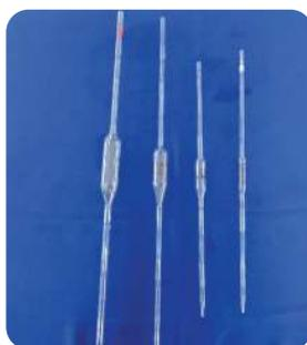
**Gambar 9.14** Pipet volumetrik (pipet gondok)
