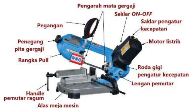
Gambar 7.45 Bagian-bagian Mesin Gergaji Pita ( Band Saw ) Horisontal.
