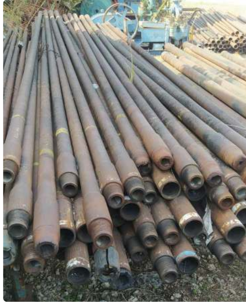
Gambar 6.20 Drill Pipe Sumber: Yudanto (2020)
