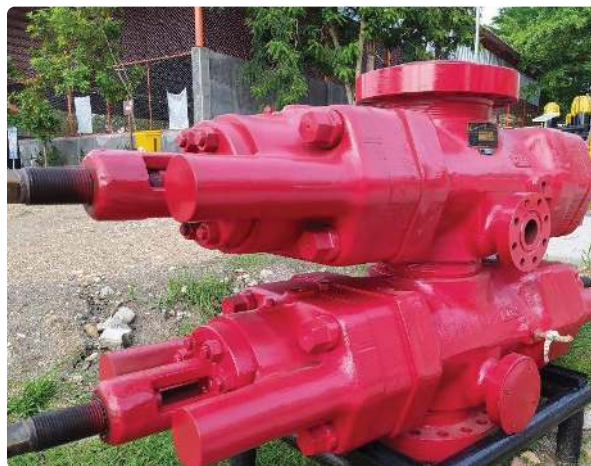
Gambar 6.27 Pipe Ram Preventer Sumber: Yudanto (2020)
