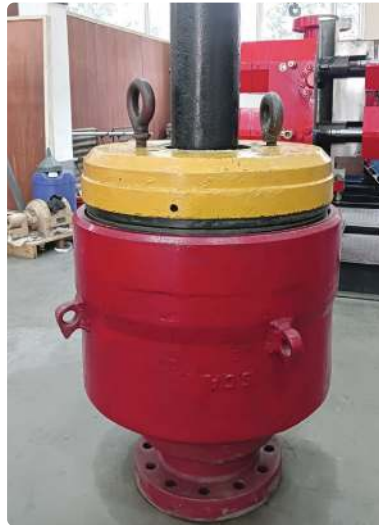
Gambar 6.26 Annular Preventer Sumber: Priyadi (2023)
