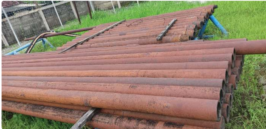
Gambar 6.21 Drill Collar Sumber: Priyadi (2023)
