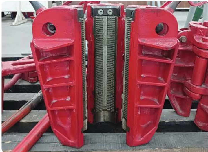
Gambar 6.17 Rotary Slip Sumber : Priyadi (2023)
