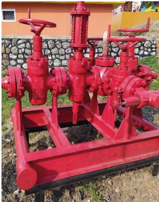
Gambar 6.29 Choke Manifold Sumber: Yudanto (2020)
