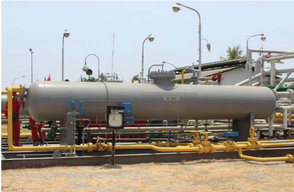
Gambar 7.26 Separator Horizontal Sumber: Yudanto (2013)
