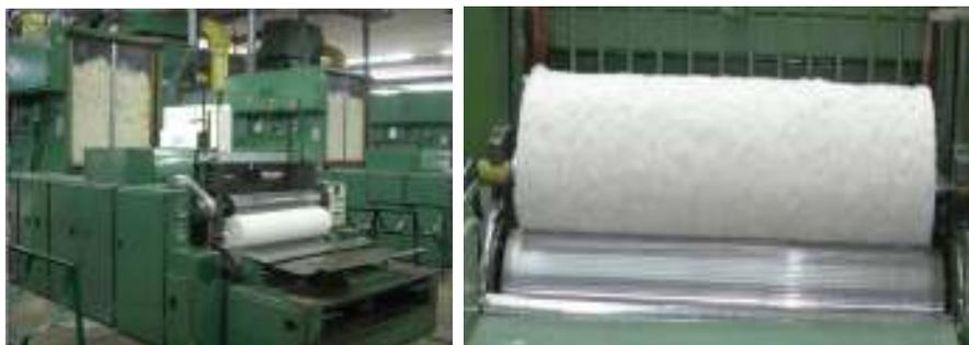
**Gambar 3.11** Mesin *Blowing*
