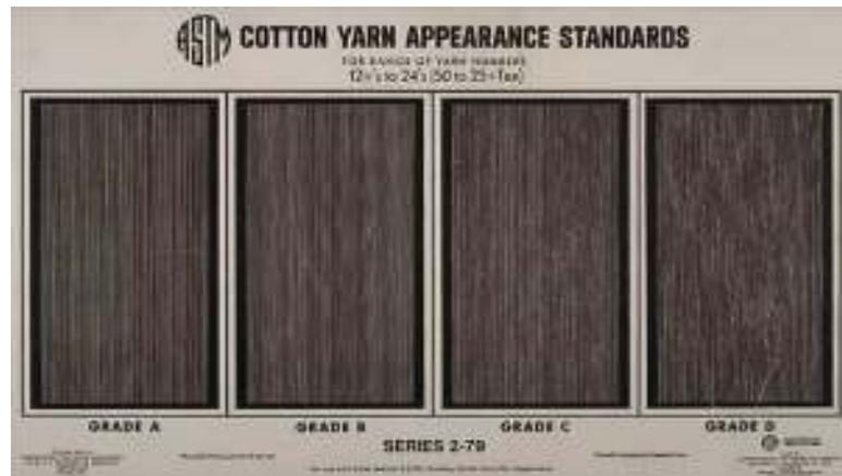
**Gambar 5.1** Standar ASTM Kenampakan *Grade* Benang
