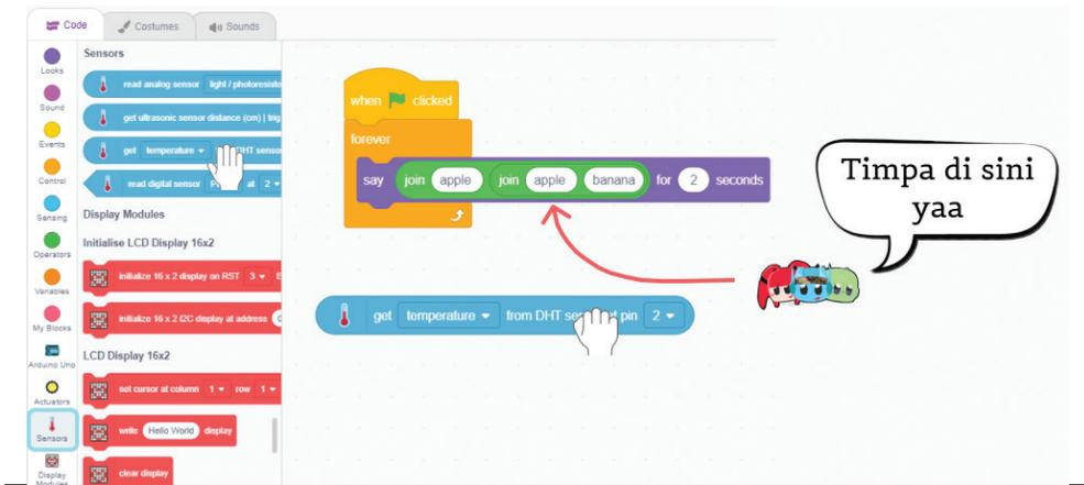
Gambar 9.32 Drag & drop blok GetTemperature (<https://s.id/GetTemperature>)
