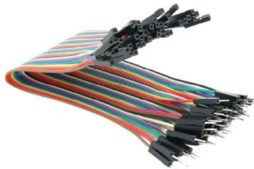
Gambar 9.16 Kabel Jumper Male to Female
