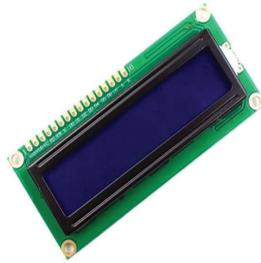
Gambar 9.20 LCD 16 x 2
