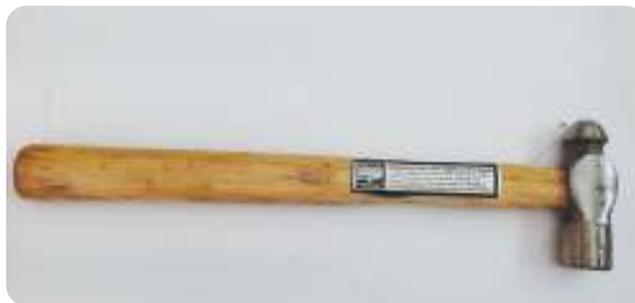
Gambar 6.18 *Ball-peen Hammer*
