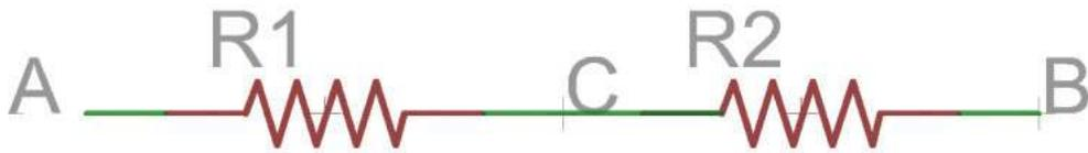
Gambar 1.7 Rangkaian Seri Resistor
