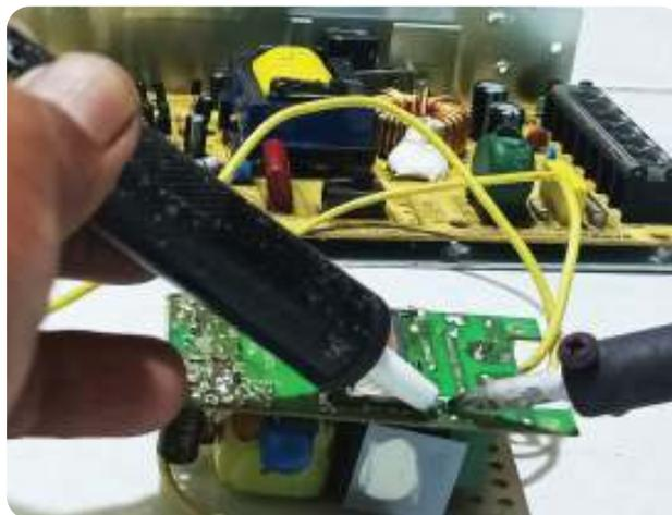
Gambar 4.6 Proses *Desoldering*
