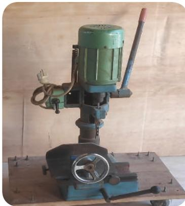
Gambar 4.51 Mesin Bor Lubang Persegi (*Hollow Chisel Mortiser*)
