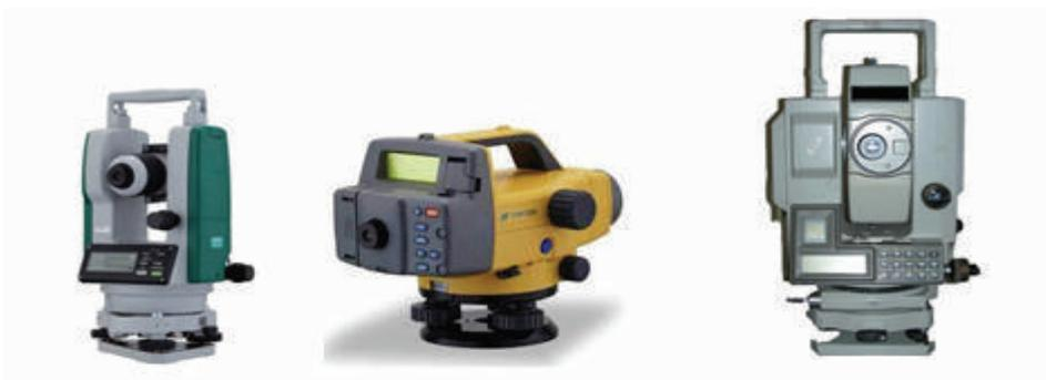
**Gambar 5.11** *Digital Theodolite*, *Digital Automatic Level*, dan *Total Station*
