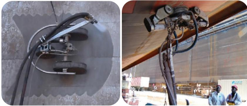
Gambar 2.19 Sandblasting Robot Mekanik
