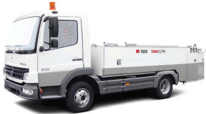
Gambar 6.85 Aircraft water service (Sumber: TIPS Ground Support Equipment, 2022)
