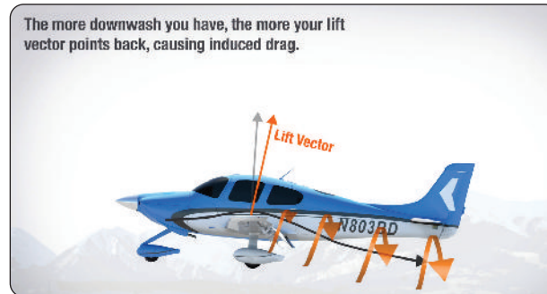
Gambar 4.31 induced drag (Sumber: boldmethod.com, 2022)
