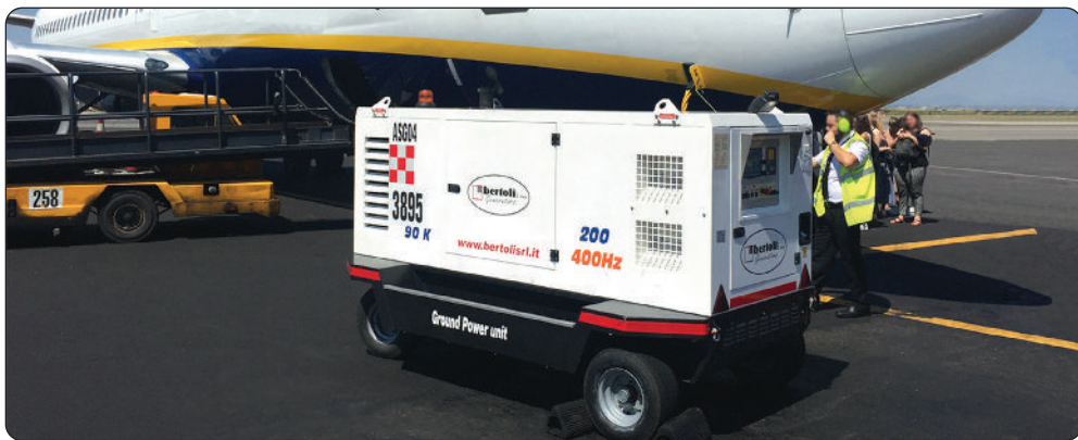
Gambar 6.88 Ground power unit saat preflight dan maintenance (Sumber: ONS Frankfurt GmbH, 2020)
