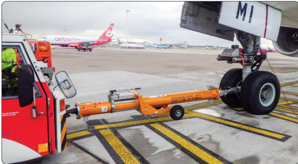
Gambar 6.90 Aircraft towing bar (Sumber: Jet Maintenance & Service, 2021)
