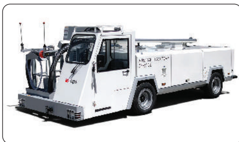
Gambar 6.86 Aircraft lavatory service (Sumber: TIPS Ground Support Equipment, 2022)
