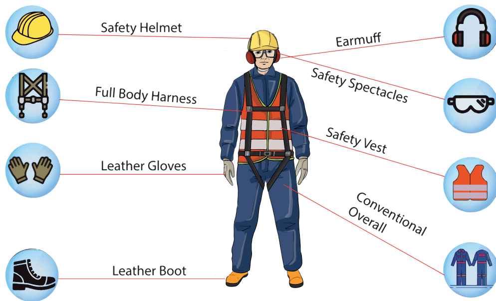
Gambar 2.3 Personal protective equipment
