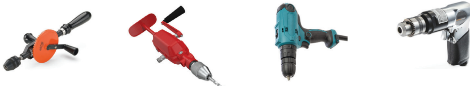
Gambar 6.61 Breast, electric, dan pneumatic drill types (dari kiri ke kanan)
